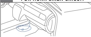
This provision permits customer connection of a switch to select either horn of siren operation when the horn pad is pressed.
