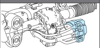
The Electric Power Steering System consists of a Rack-and-Pinion steering gear assisted by an electronically controlled power steering motor and drive assembly.
