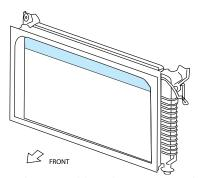
Transmission oil is pumped from the transmission through piping to an oil to air heat exchanger in the upper portion of the air conditioning condenser tuning and returns to the transmission. The air conditioning condenser is located in front of the engine coolant radiator as part of the Cooling Fan and Radiator Module (CFRM) assembly.
