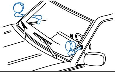
Spotlamp left hand, pillar-mounted unity, 6-inch with replaceable H3 halogen bulb; independently fused
