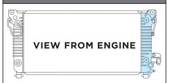
Engine Oil and Transmission Oil are cooled by passing the fluids through separate coolers located in the engine radiator assembly end tank and the air conditioning condenser.
