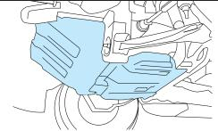
Two piece aluminum front underbody shield staring behind the front bumper and running to the 2nd cross-member protecting front underbody and oil pan.
