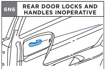
Rear door locking rods are disabled. Rear door locks are inoperable at rear doors, but operate from driver position. Inside rear door handles are disconnected. Rear doors can only be opened from the outside.
