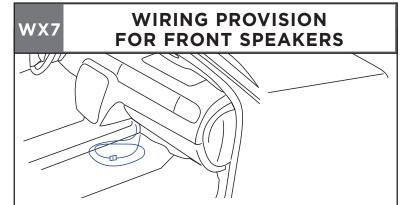
Approximately 60 inches (1.5 m) of auxiliary speaker wiring is routed from the front door and windshield pillar speakers and coiled under the instrument panel. The wiring permits connection of the front speaker pairs to customer-installed communication equipment. Vehicle radio front speaker outputs are re-routed to the rear speakers to maintain the required open door/key-inignition and other audible warnings.
