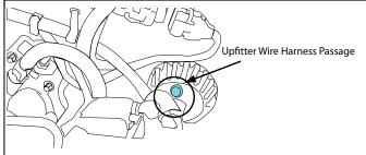
Provides pass through for small number of wires and is located at the lower left side of the front of dash. Carefully remove or puncture only the nipple portion for passage of wire and silicone seal around the wire after installation. Note that a vehicle harness connector is located at the interior side of the grommet and may interfere with passage of wire.
