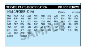
A Service Parts Identification (SPID) Label provides Vehicle Identification Number (VIN)-specific Option Code content list, Engineering Model Number (Nameplate, body style), Exterior paint system, Exterior paint color code and Interior trim level and color. The SPID label for the Tahoe is located on the inner surface of the instrument panel storage compartment (glove box).
