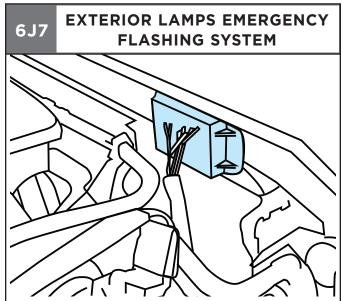
Option 6J7 provides a headlamps high beam flashing module, rear lamps flashing via the Body Control Module (BCM) and a control wire for customer-furnished switching to turn the module on and off. The flasher control wire is part of the blunt-cut upfitter harness coiled under the instrument panel in the front passenger side foot well. The flashing module is located on the rear edge of the right hand upper radiator support.
